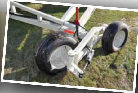
Walking axle reduces uneven terrain by half
